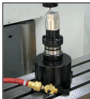
2 3 / 16 -10 threaded-nose accepts collets, expanding collets (shown), step chucks and manual chucks.
