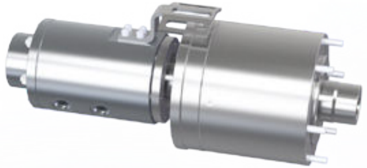
Hydraulic thru hole cylinder with triple passage rotary air coupling mounted for air sensing, anti-vibration arms and work support units
