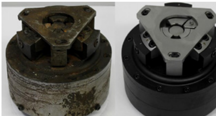
7" 3 Jaw Diaphragm Chuck Assembly with Special Tooling
